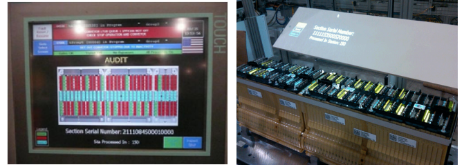
(a) Initial display for presenting “suspect” weld positions to the human inspector. “suspect” welds are highlighted in red color. (b) Projected light on battery section highlights “suspect” welds for manual inspection.
