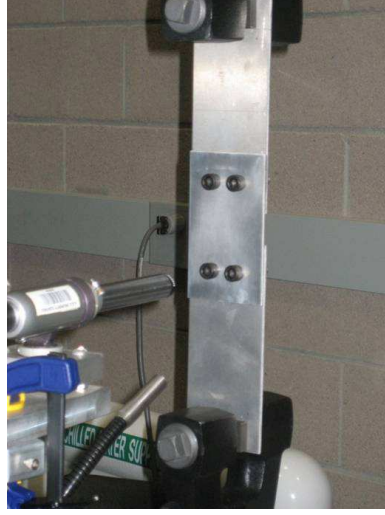
Fig. 4.2. Setup for structural and material damage in a bolted joint.
